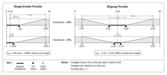
Fig. 9 Effect of adjusting the throttle deadband parameter.
