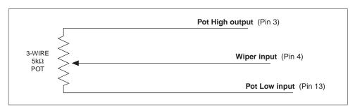
For wigwag and inverted wigwag applications, the pot can be correctly centered within the controller's neutral band by using the throttle autocalibration feature (see page 23). Pots with less than 5 k $\Omega$  total resistance change over the throttle's full stroke can be accommodated by programming the controller for reduced-range throttle inputs, via the throttle gain parameter (see page 25).
