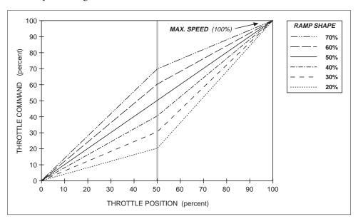
Changing the maximum speed setting changes the throttle command range, and hence the ramp shape. Ramp shapes with the maximum speed setting dropped from 100% to 60% are shown in Figure 12.
