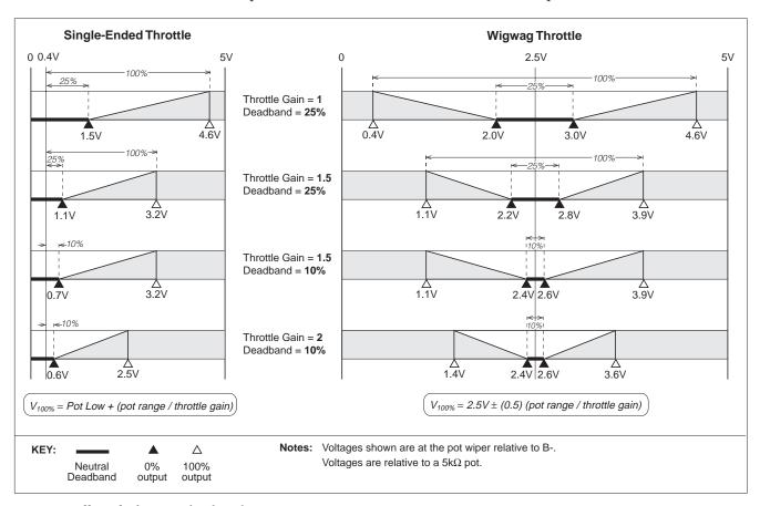
**Fig. 10** *Effect of adjusting the throttle gain parameter.*
