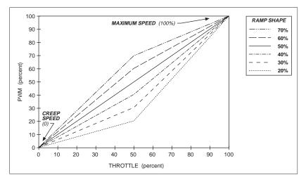
Changing either the maximum speed setting or the creep speed setting changes the output range of the controller. Ramp shape output is always a percentage of that range. Ramp shapes with the creep speed setting raised to 10% are shown in Figure A-2. In Figure A-3, the creep speed is kept at 10% and the maximum speed setting dropped to 60%.
