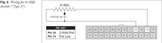
With Type 3 throttles, broken wire protection is provided by the controller sensing the current flow from the 2-Wire Pot pin through the pot and into the Pot Low pin. If the Pot Low input current falls below 0.1 mA, a throttle fault is generated and the controller is disabled. NOTE: The Pot Low pin (Pin 14) must not be tied to ground.
