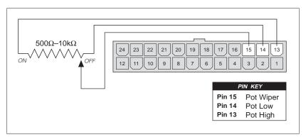
As with the 2-wire throttles, broken wire protection is provided by the controller looking for a minimum current into the Pot Low pin. If the Pot Low input current falls below 0.1 mA, a throttle fault is generated and the controller is disabled. NOTE: The Pot Low pin (Pin 14) must not be tied to ground.
