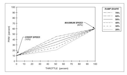
In all cases, the ramp shape number is the PWM output at half throttle, as a percentage of its full range. So, for example, in Figure A-3, a 50% ramp shape gives 35% PWM output at half throttle (halfway between 10% and 60%). A 30% ramp shape gives 25% PWM at half throttle (30% of the range {which is 50%, from 10% to 60%}, starting at 10% output, or  $\{[.30 \times 50\%] + 10\%\} = 25\%$ ).
