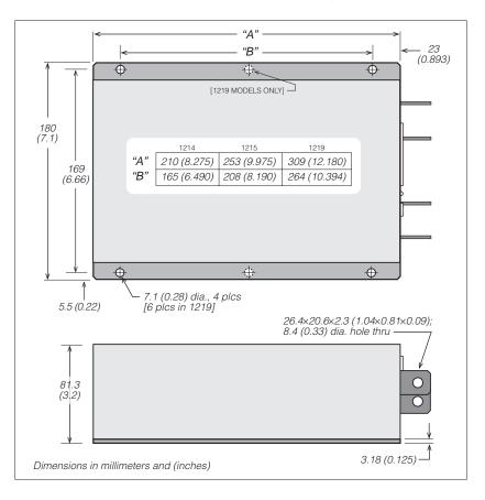
Fig. 2 Mounting dimensions, Curtis 1214-/15-/19-8 controllers.
