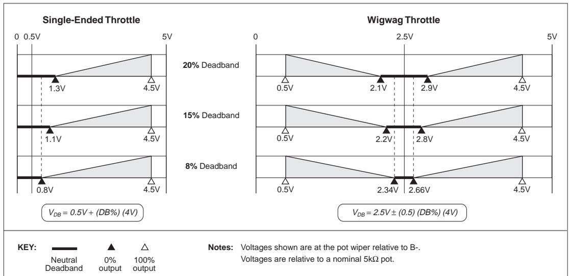
**Fig. 20** Effect of adjusting the neutral deadband parameter.
