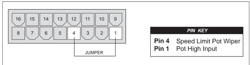
If a speed limit pot will never be used in the application, the controller can be factory-configured without the speed limit feature (see Section 4), and the jumper will not be required. With such a controller, the vehicle speed at full throttle is defined by the programmed maximum speed, and it is possible to program the reverse speed to a lower value if so desired.
