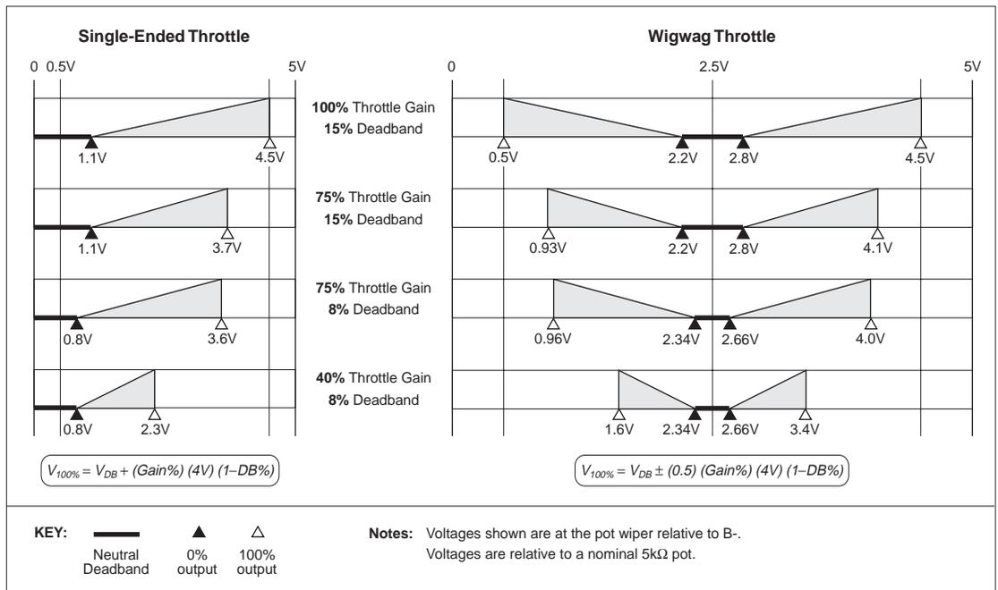
Fig. 21 Effect of adjusting the throttle gain parameter.
