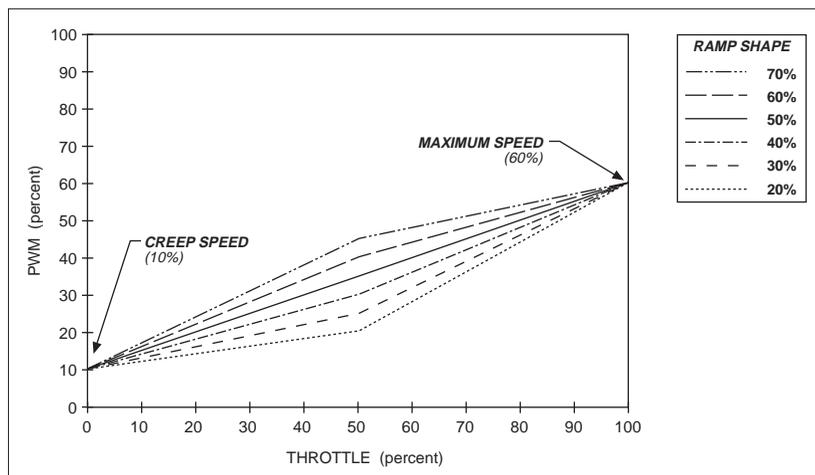
In all cases, the ramp shape number is the PWM output at half throttle, as a percentage of its full range. In Figure 24, for example, the 50% ramp shape gives
