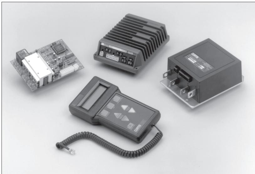
The 1223/33, 1225/35, and 1227/37 MultiMode™ controllers offer smooth, silent, cost effective control of motor speed and torque. A four quadrant, full bridge power output stage provides for solid state motor reversing and full braking power without additional relays or contactors.
