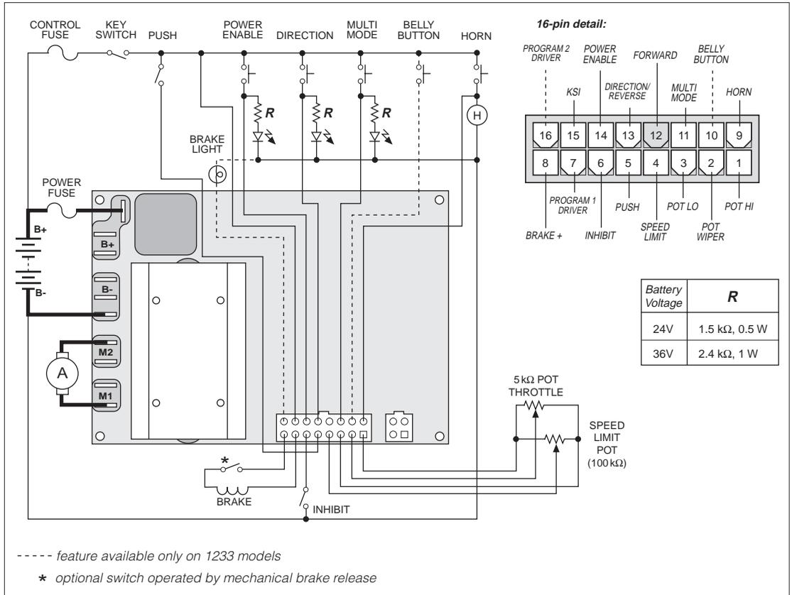
**Fig. 4** Basic wiring configuration using momentary switches, Curtis PMC 1223/33 controller.
