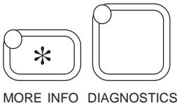
In the **Special Diagnostics** mode, the controller’s diagnostic history file is displayed. This file includes a list of all faults observed and recorded by the controller since the history was last cleared. (NOTE: The maximum and minimum temperatures recorded by the controller are included in the Test Menu.) Each fault is listed in the diagnostic history file only once, regardless of the number of times it occurred.
