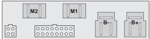
Mating connectors are available. The 3-terminal battery connectors are Curtis PMC p/n 16551, and the 2-terminal motor connectors are p/n 16552. Both connectors use Curtis PMC p/n 16553 terminal pins designed for use with #10 AWG (2.59 mm).
