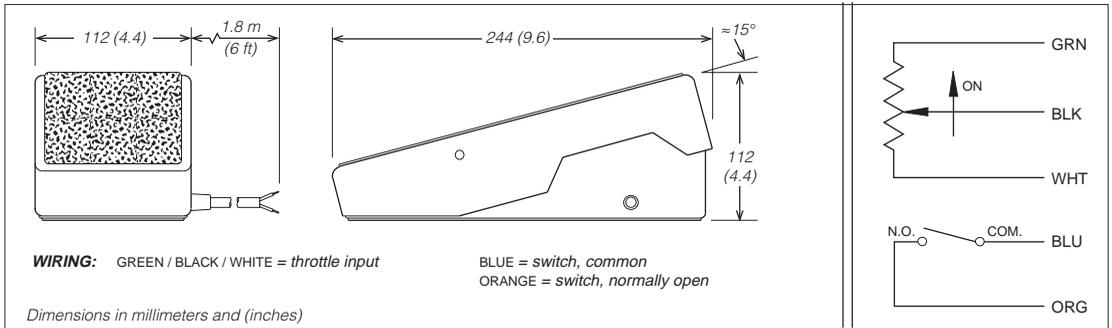
**Fig. B-4** Mounting dimensions, Curtis electronic throttle (ET series).
