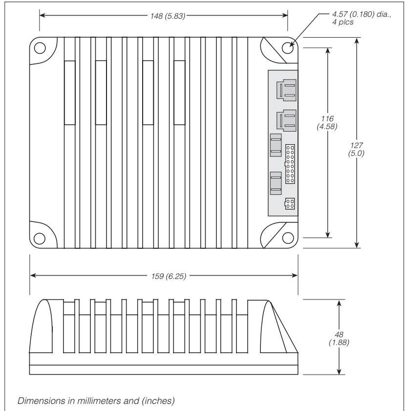
The 1225/35 controller can be oriented in any position. To ensure full rated output power, the controller should be positioned so that the maximum available airflow travels across its ribs. Fasten the controller to a secure mounting bracket or other surface, using the four mounting holes provided. Be sure to allow easy access to the controller's connection face so that the 1307 handheld programmer can be plugged into the controller after it is installed.
