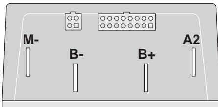
Cables are fastened to the bus bars by M8 ( $\frac{5}{16}$ " ) bolts. When tightening the bolts, two opposing wrenches should be used to prevent bending the bus bars and putting undue strain on the internal connections.
