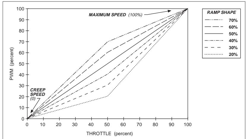
Changing either the maximum speed setting or the creep speed setting changes the output range of the controller. Ramp shape output is always a percentage of the output range (the range between the creep speed and maximum speed settings).
