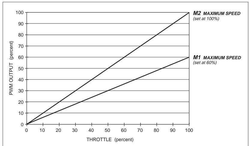
The speed interlocks (see Section 4) ensure that Mode 2 is by definition the faster of the two modes. The M1 Maximum Speed cannot be set higher than the M2 Maximum Speed.
