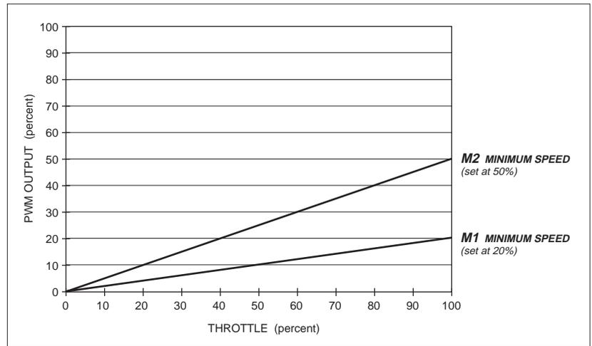
The speed interlocks (see Section 4) ensure that the minimum speed is set lower than the maximum speed in each mode (M1 Min Speed < M1 Max Speed, and M2 Min Speed < M2 Max Speed).
