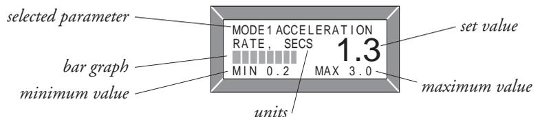
Some parameters on some controllers have dependencies on other parameters. This means that the available settings for one parameter may be dependent on the limits of another parameter. For example, your controller may not allow the reverse speed to be set below the Mode 1 minimum speed. In this example, if you attempt to reduce the reverse speed below the M1 minimum speed, a message will be displayed indicating that the minimum reverse speed is dependent on the M1 minimum speed.
