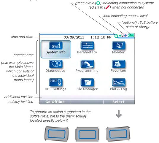
In this example, pressing the "Select" softkey will open the System Info menu, which is highlighted. The "Select" softkey opens whichever menu is highlighted. Pressing the "Offline" softkey allows you to use the programmer when it is not connected to a controller; see Section 15.
