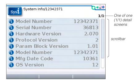
The sliding bar at the right of the screen indicates there are more items than those shown. Use the down-arrow key  $(\nabla)$  to scroll down to see the rest of the list.
