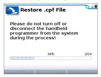
There may be a series of these progress bars. Above the right end of the progress bar you will see a number; in this example, the number "2/14" is telling you this is the second of fourteen progress bars.
