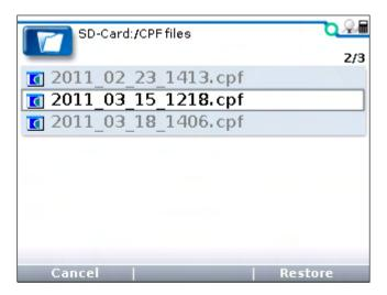
After you highlight a .cpf file and choose "Restore," a pop-up screen will ask whether you want to enable Advanced Cloning ("yes"/"no"). This screen does not appear on User-level and Service-level programmers.
