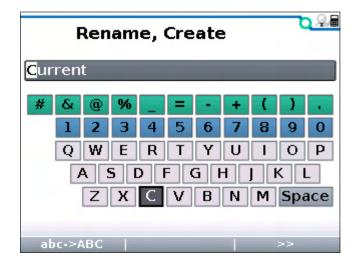
Use the four arrow keys to move around the keyboard—up, down, right, and left. In the text line, use the "+" key (+) to move the highlight one space to the right, and the "-" key (-) to move the highlight one space to the left.
