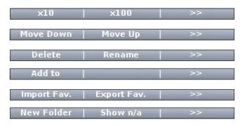
You can change the settings of your Favorite parameters while you are in the Favorites menu; it is not necessary to be in the Parameters menu to do this. The " $\times 10$ " or " $\times 100$ " softkey, pressed together with the "+" or "-" key, allows you to change values rapidly.
