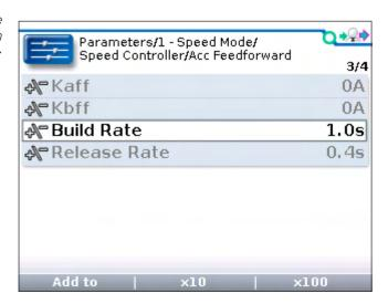
the Speed Mode folder is highlighted, the "×10" and "×100" softkeys are grayed out (indicating they do not apply)—but when Build Rate is highlighted, these softkeys are available.
